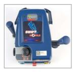
The machine is operated by a 2900 mAh, rechargeable battery. When the machine is fully charged it can duplicate up to 100 brass keys. Coloured light indicators show the level of the battery and when it needs recharging.
